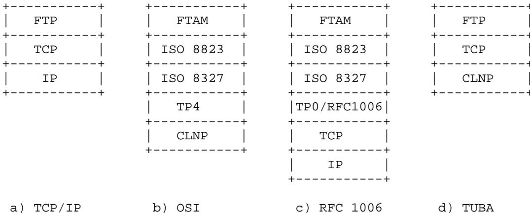
Figure 2: Protocol stacks providing file-transfer service.
