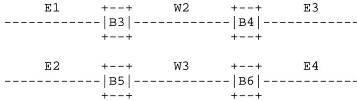
To accomplish this (using the LAN Identification option), B1 and B2 negotiate this option on, and send datagrams with bit 6 set to 1, with the LAN ID field inserted in the frame. Traffic on E1 and E3 would be assigned LAN ID 1, and traffic on E2 and E4 would be assigned LAN ID 2. Thus B1 and B2 can separate traffic going over W1.
