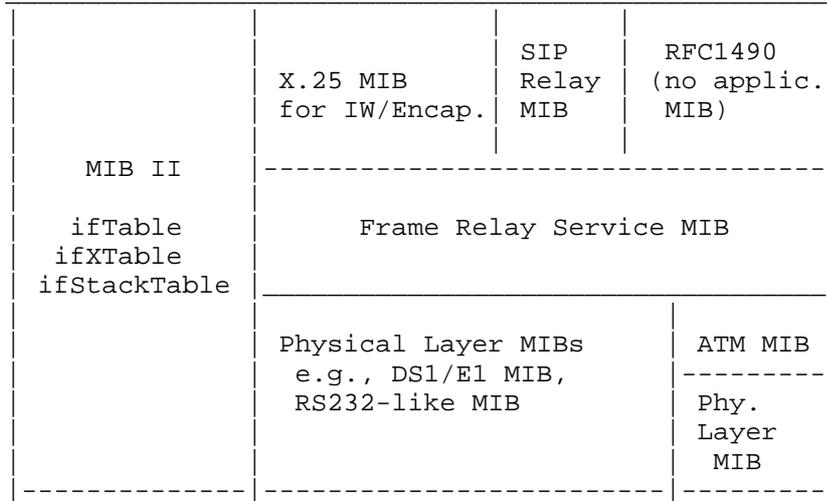
Figure 1. Frame Relay MIB Architecture
