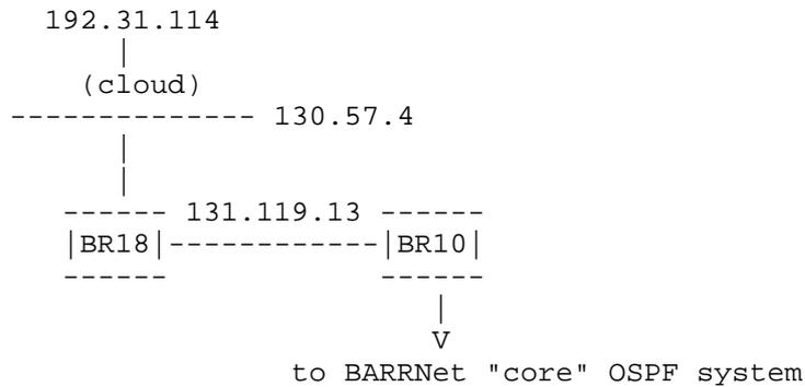
where the "cloud" consists of the subnets of 130.57 and network 192.31.114, all of which are learned by RIP on router BR18. Topologically, this cloud looks very much like an OSPF stub area. The advantages of running the cloud as an OSPF stub area are:
