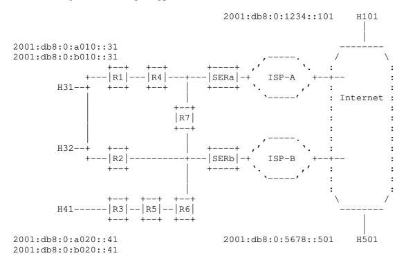
Figure 2: Simple ISP Connectivity Where SERs Are Not Directly Connected
