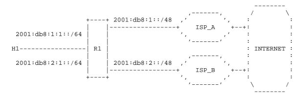
Figure 1: Single Router, Primary/Backup Uplinks
