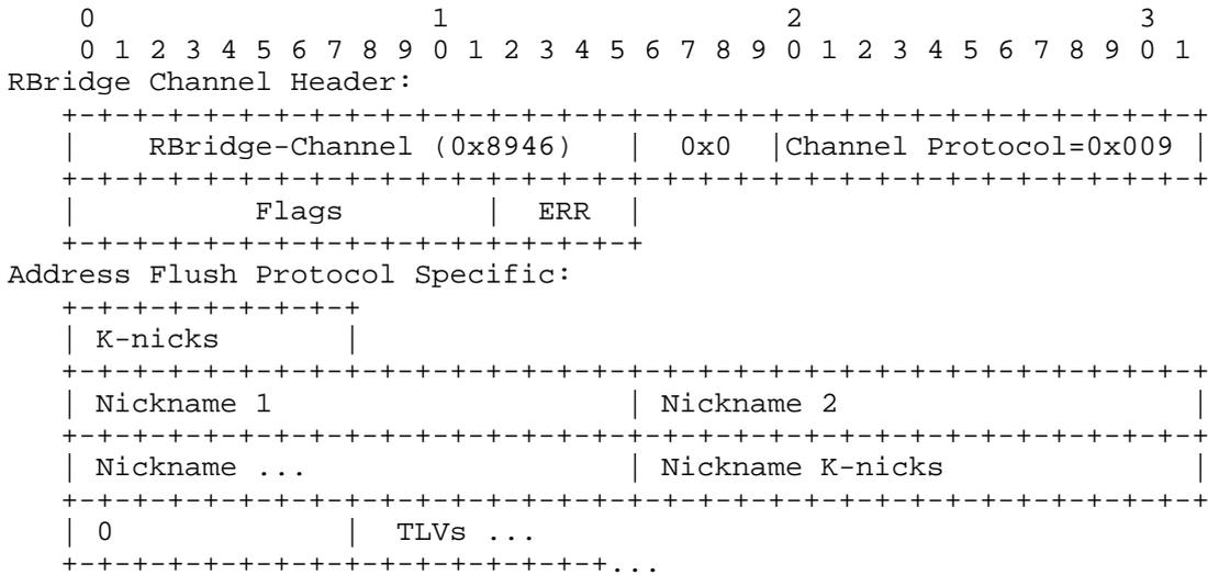
Figure 3: Address Flush Message - Extensible Case
