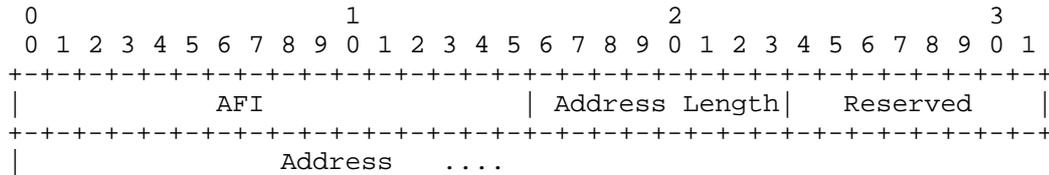
Figure 2: Interface Identification Object - C-Type 3 Payload
