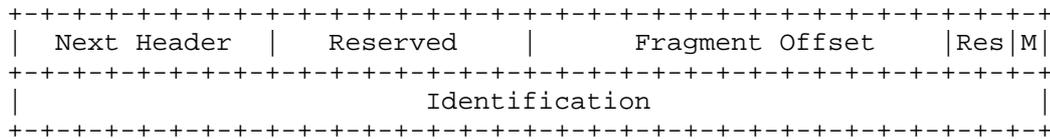
Next Header            8-bit selector. Identifies the initial header type of the Fragmentable Part of the original packet (defined below). Uses the same values as the IPv4 Protocol field [IANA-PN].
