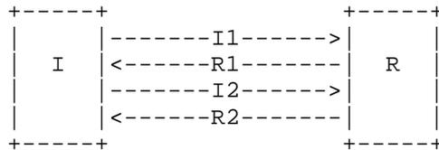
Figure 1: HIP Base Exchange without a Rendezvous Server
