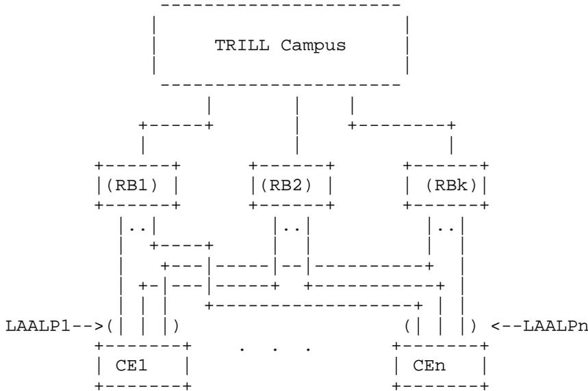
Figure 1: Active-Active Connection to TRILL Edge RBridges
