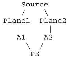
Figure 2: PE is Dual-Homed to Dual-Plane Backbone
