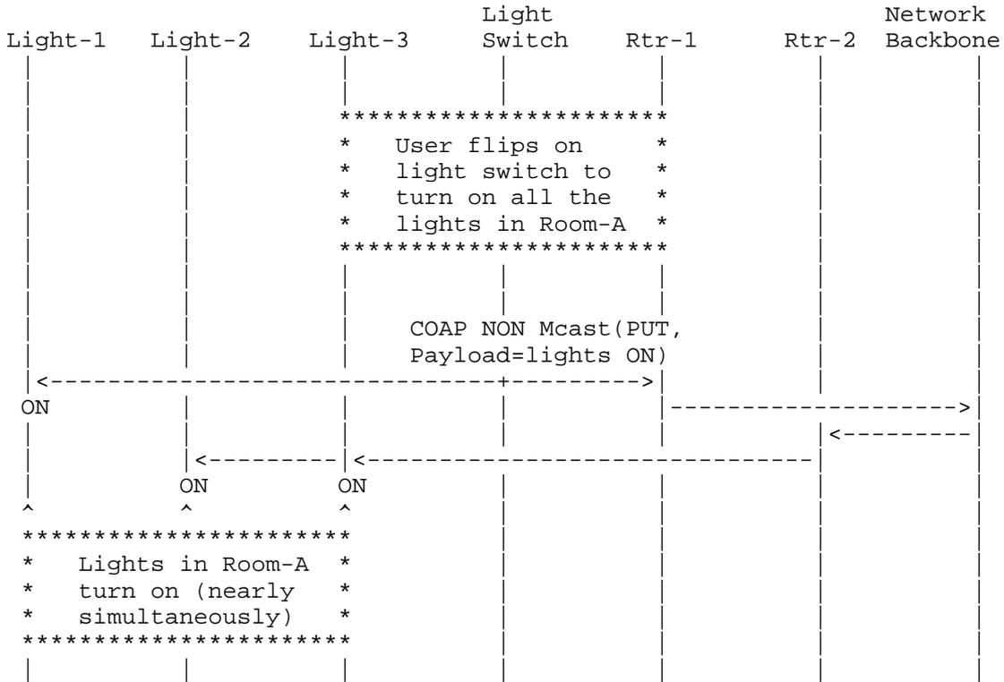
Figure 3: Light Switch Sends Multicast Control Message
