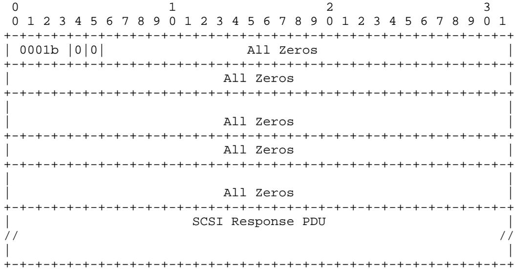
Figure 10: iSER Header Format for SCSI Response PDU
