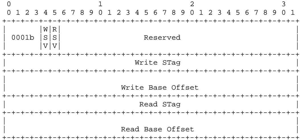
Figure 3: iSER Header Format for iSCSI Control-Type PDU
