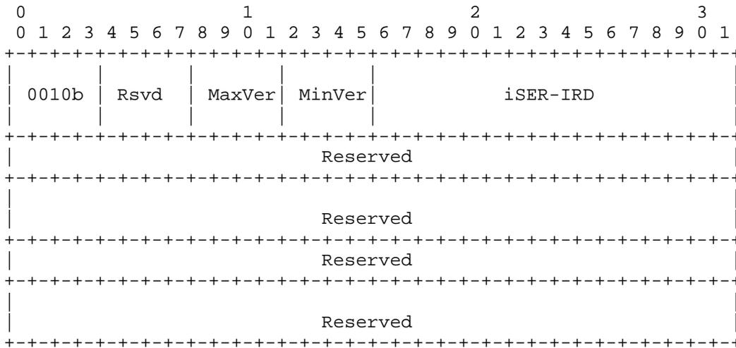
Figure 4: iSER Header Format for iSER Hello Message
