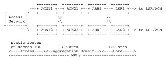
Figure 1: Seamless MPLS End-to-End Reference Network Topology
