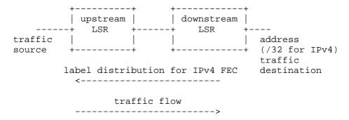
Figure 7: LDP Label Assignment Direction
