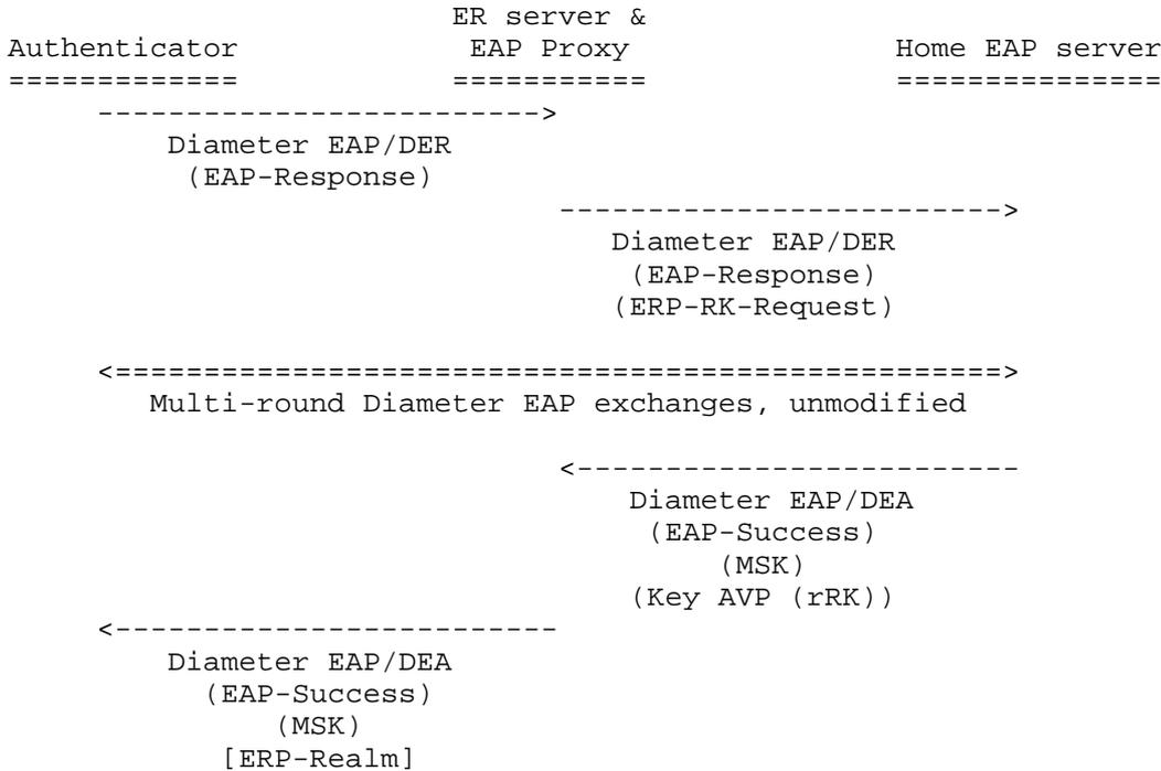
Figure 2: ERP Bootstrapping during Full EAP Authentication
