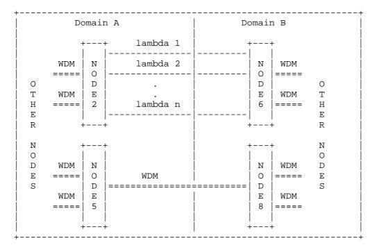
Figure 2. Interconnecting Details between Two Domains
