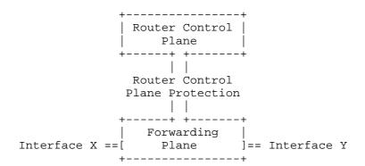
Figure 1: Router Control Plane Protection
