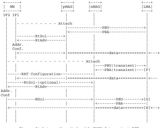
Figure 6: Late path switch with PMIPv6 transient BCEs
