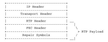
Figure 6: Format of repair packets
