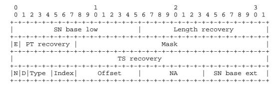
Figure 7: Format of the FEC header
