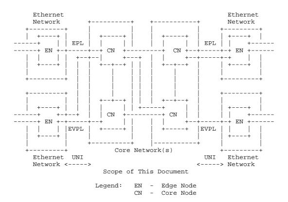
Figure 1: Ethernet UNI Reference Model
