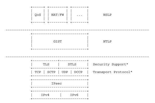
\* The Security Support and Transport Protocol layers show some possible protocols that could be used to transport NSIS messages. To provide authentication and/or integrity protection support, the transport protocol has to be paired with a suitable security mechanism, e.g., TCP with TLS, or Datagram Congestion Control Protocol (DCCP) with DTLS.
