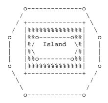
Figure 5: Hole with Enclosed Polygon (Island)
