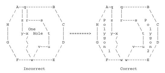
Figure 4: Specification of Hole with Multiple Outer-Boundary Intersections
