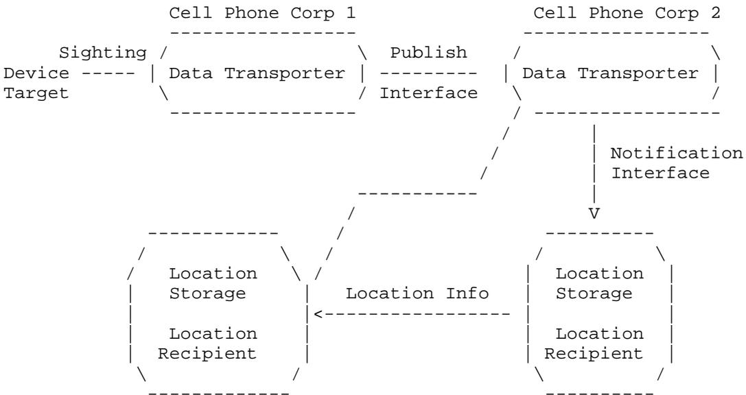
Here, cell phone Corp 1 is the AP and the LG. In this scenario, Cell phone Corp 2 is likely to be a Trusted entity, but cell phone Corp 1 may be Non-trusted.
