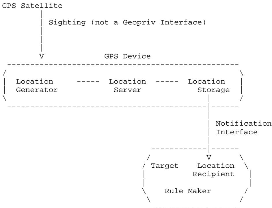
In this scenario the GPS Device is both the AP and the LG. The interaction occurs in a Trusted environment because it occurs in the Rule Maker's Device.
