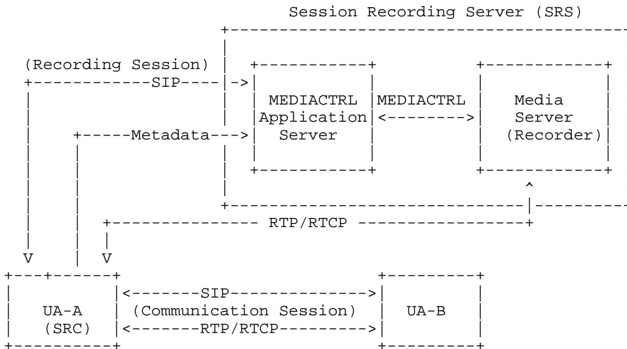
Figure 3: Example of Session Recording Server using MEDIACTRL
