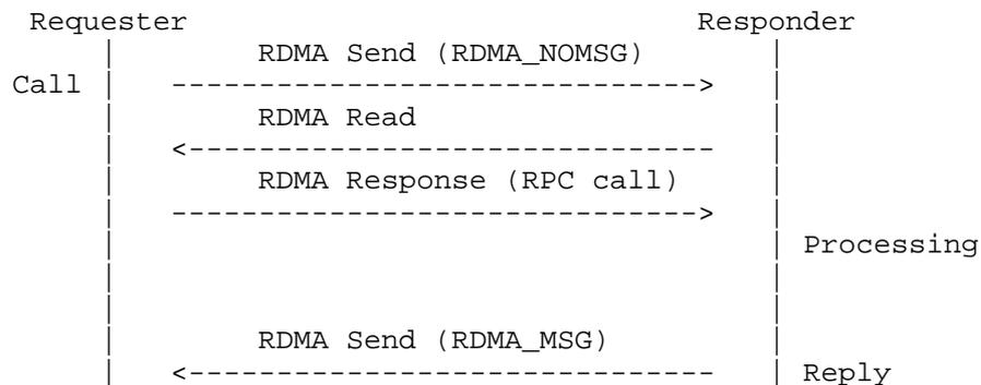
An RPC-over-RDMA transaction using a Long Reply:
