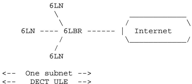
Figure 5: DECT ULE network connected to the Internet
