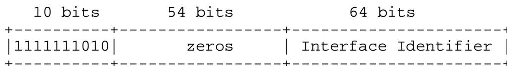
Figure 4: IPv6 link-local address in DECT ULE
