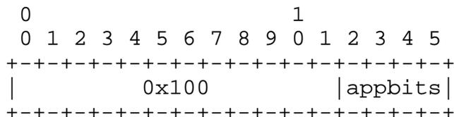
The appbits field is 4 bits that are application-dependent and may be defined to be any value or meaning, and are outside the scope of this specification. For the purposes of signaling, this field is treated as a special extension value assigned to the local identifier 256. If no extension has been specified through configuration or signaling for this local identifier value 256, the appbits field SHOULD be set to all 0s by the sender and MUST be ignored by the receiver.
