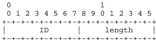
The 8-bit ID is the local identifier of this element in the range 1-255 inclusive. In the signaling section, the range 1-256 is referred to as the valid range, with the values 1-255 referring to extension elements, and the value 256 referring to the 4-bit field 'appbits' (above).
