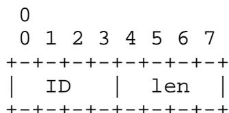
The 4-bit ID is the local identifier of this element in the range 1-14 inclusive. In the signaling section, this is referred to as the valid range.
