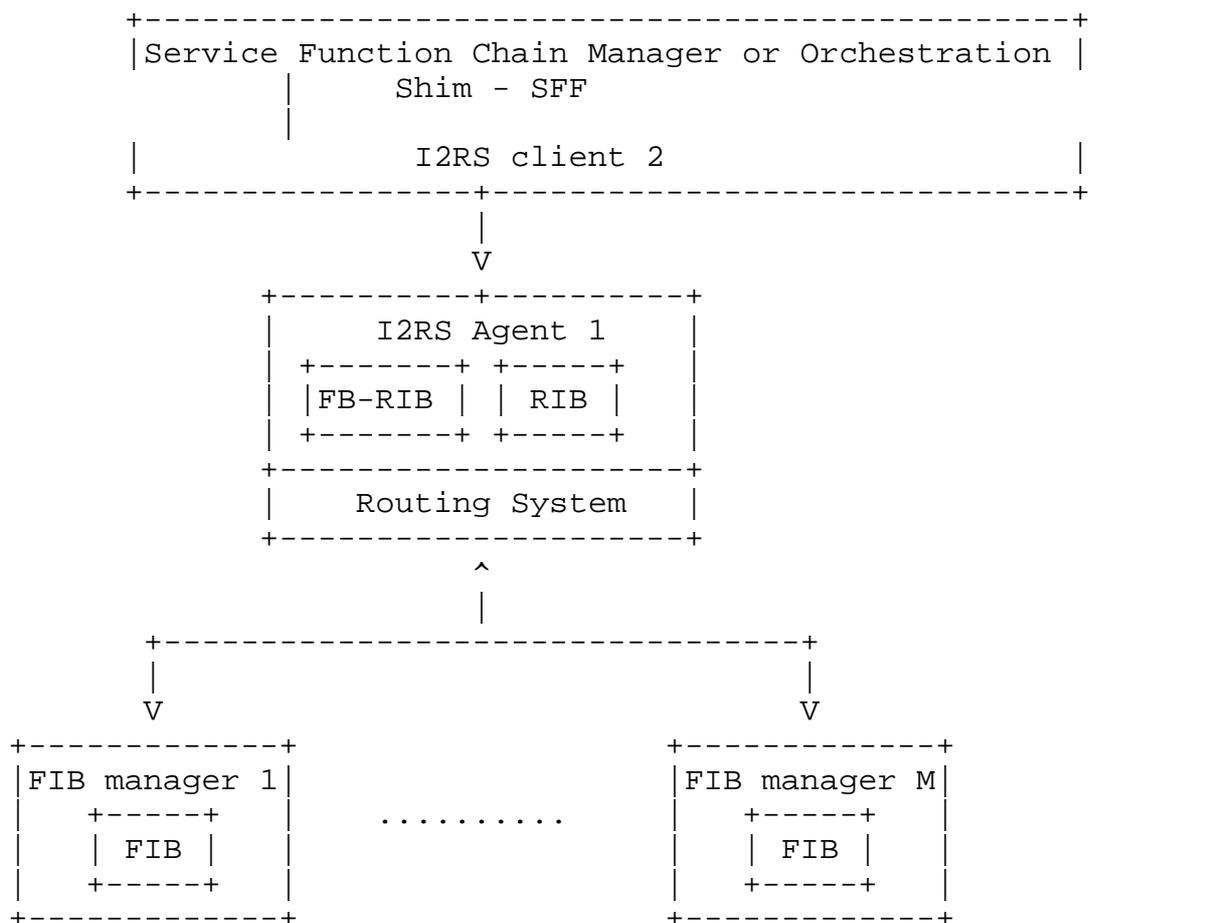
Figure 2 SFF Shim Layer in relation to RIB Manager
